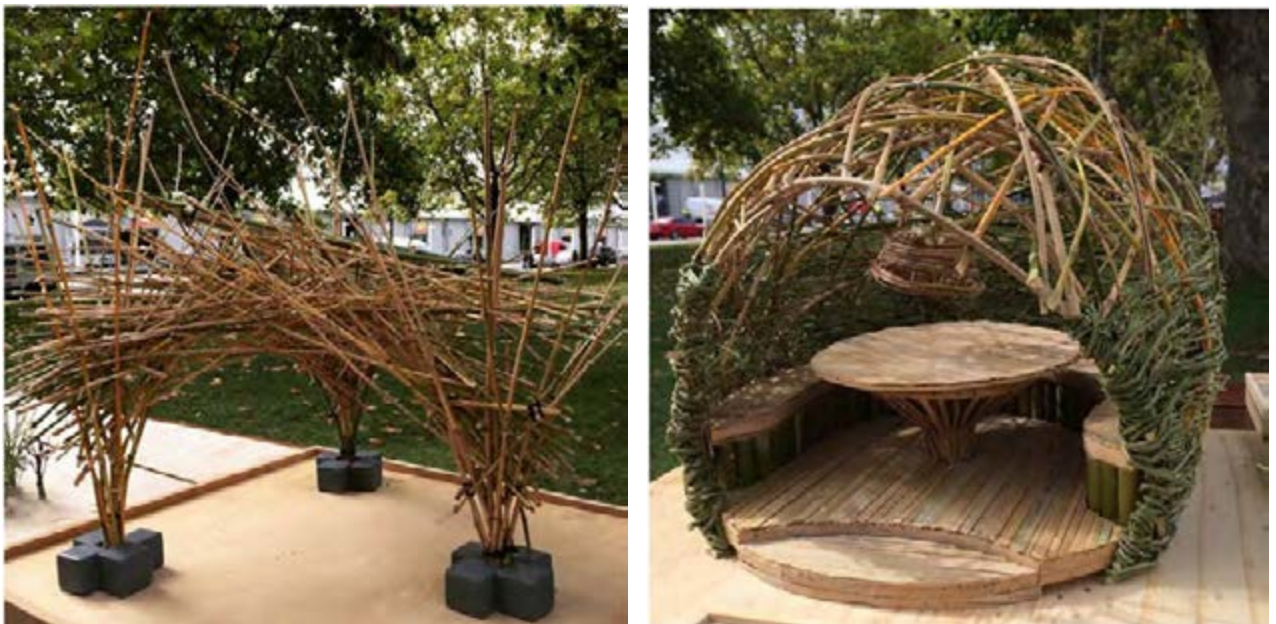
Figure 2: Scale models of structural bay of canopy (left) and pods (right) Images: Helen Norrie.
